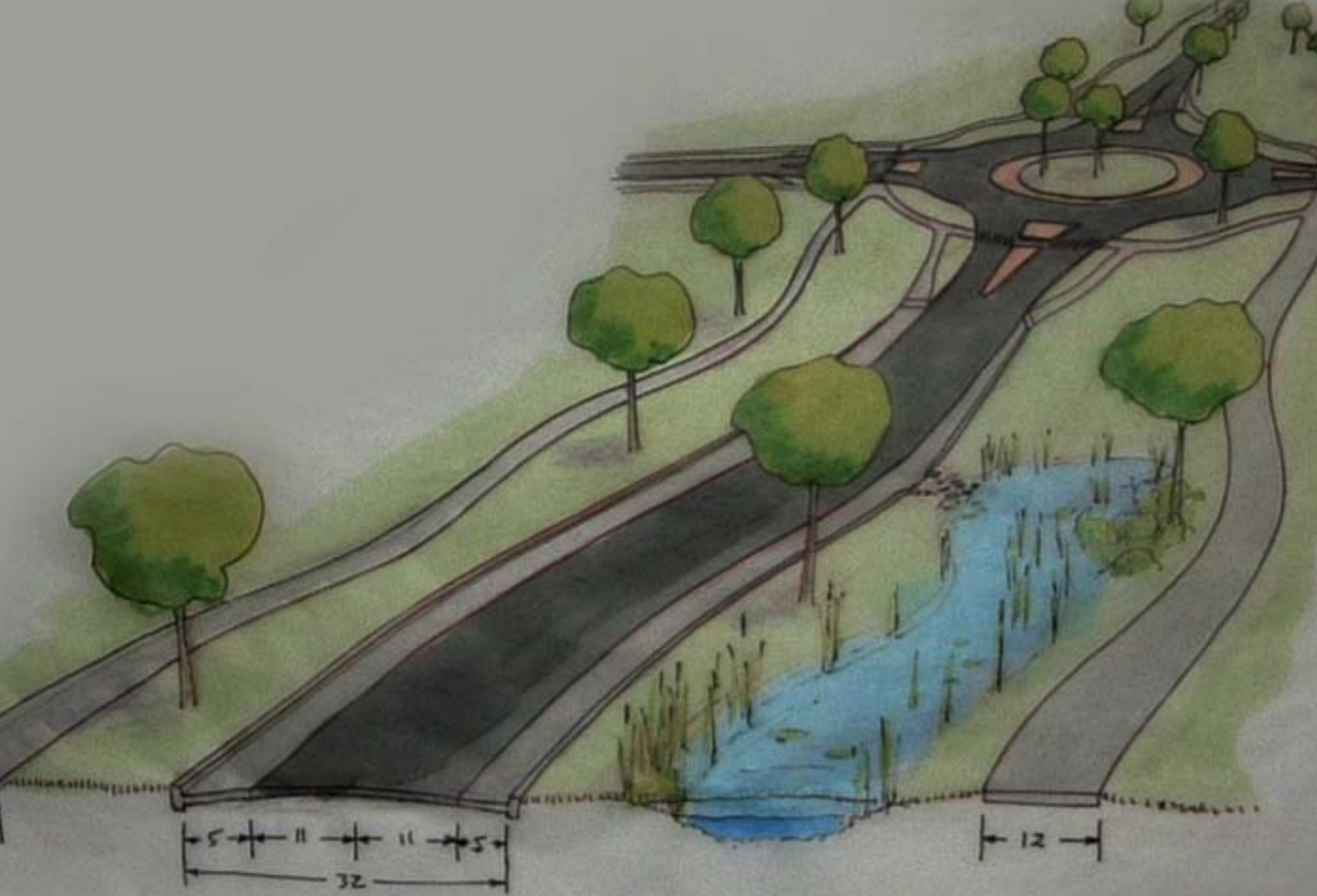
SOUTH BRANCH PARKWAY CROSS-SECTION
